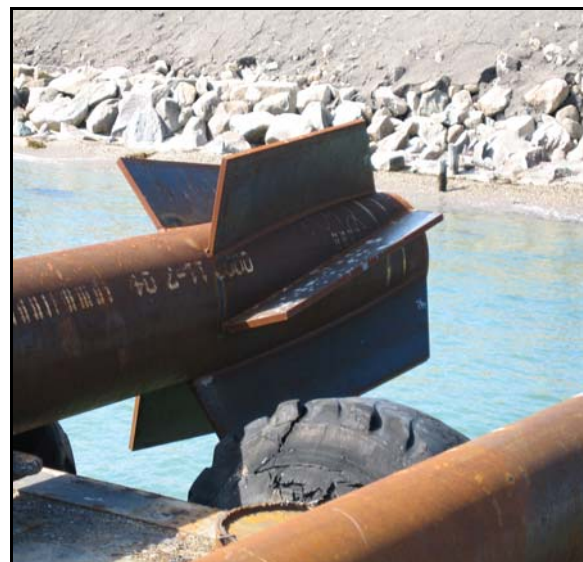
Figure 1. Typical Spin Fin® pile.
