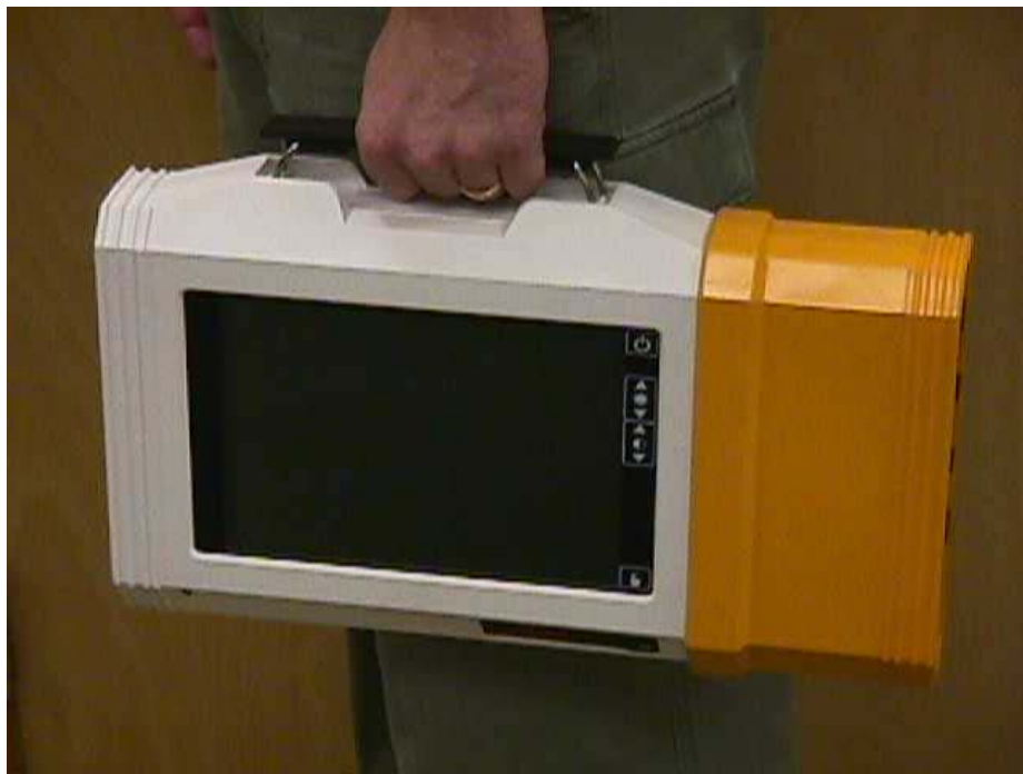
Figure 5 Photograph of the Pile Integrity Sonic Analyzer (PISA)
